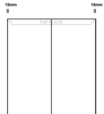
**Standard Shed — Bottom Plate will protrude below wall sheet by approximately 10mm.**
